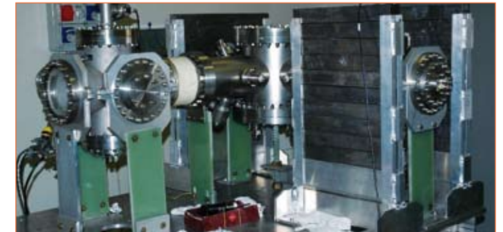
1. Inside this vacuum chamber an electrostatic optics collects the positrons emitted by a radioactive source (on the right in the photography, just behind the lead shields) and focalizes them on a target (on the left in the photography)
