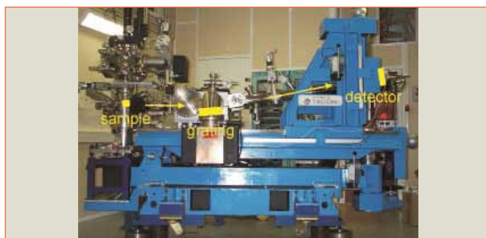
1. The AXES spectrometer at the ID08 beamline of the ESRF
