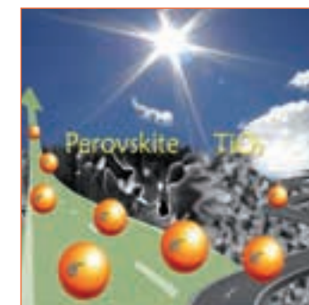
1. Cartoon illustrating the double path for electrons percolation in mesostructured PSC, with slow and fast dynamics associated to \text{TiO}_2 and perovskite transport respectively, hypothesized according to TCSPC, cw-PIA and TPV analysis.
